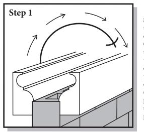
**Step 1.** Wall Cap Form installation is a two person job, having one person on each side of the wall. Place the Wall Cap Form on the top of the wall with the lip of the form resting on top of the wall (this will position the form to elevation). With each person holding the form in place, the first person inserts one side of the spring clamp in place (holding firmly). The second person pulls the other side of the spring clamp up and over the second form and positions the spike in place.
