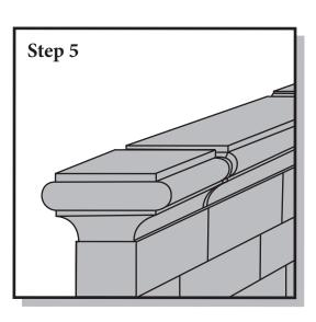
**Step 5.** Once the concrete can support its own weight, the forms should be removed. Remove the spring clamps and pull the form down and away, exposing the face for finishing.
