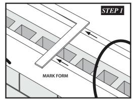
**Step 1.** Using a framing square, mark the location of the joints to be tooled.
