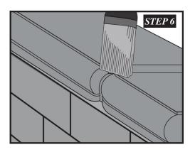
**Step 6.** Joints may be finished with a damp brush if desired.
