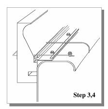
Note: The tie wires can be fastened one of two ways. They can be wrapped around the back lip of the wall or you can use the other (100) self tapping screws. To use the screws, just fasten them 4" behind the plumb strip (only half way down and wrap the tail of the tie wire around them.
