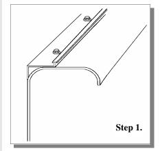
**Step 1.** Lay the plumb strip level on the edge of the wall. Use (100) screws to fasten down the strip. Fasten the strip down with self tapping screws every 8". Butt the strips up tightly as they will be showing after the job is complete.
