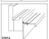
**STEP 6.** Peel the paper from the double-faced tape on the face form 1 foot at a time. Line the bottom of the face form up with the bottom of the extender. Press the face form to the extender.
