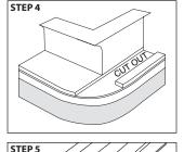
**STEP 4.** Place the preformed corners in the corners of the pool on the opposite end of the roller. The cut out in the corners should run parallel with the track side (see illustration). Peel the paper from the double-faced tape one side at a time. Line up the groove of the corner with the top lip of the liner track. Press the form to the pool wall.
