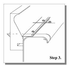
Note: The tie wires can be fastened one of two ways. They can be wrapped around the back lip of the wall or you can use the other (100) self tapping screws. To use the screws, just fasten them 4" behind the plumb strip (only half way down and wrap the tail of the tie wire around them.
