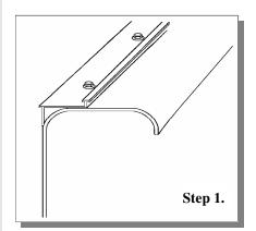
**Step 1.** Lay the plumb strip level on the edge of the wall. Use screws to fasten down the strip. Be sure to butt the joints tightly together as the strip will be visible in the finished product.
