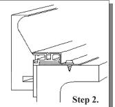
**Step 2.** Peel the paper off the double faced tape (one foot at a time) to attach the form. Insert the rib of the form into the track and stick the form to the pool wall.
