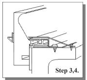
**Step 3.** Drive the concrete nails into the bond beam approximately 12" apart.
