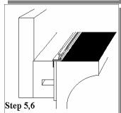
**Step 6.** Cover the top of the bond beam with 15 lb. felt to act as a "bond breaker", allowing the concrete deck to expand and contract without disturbing the tile.
