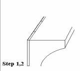
**Step 1.** Tile must be set from the high point of the bond beam and bedded out level. Scrape the top of the tile to remove any debris that would cause the tile strip to fit unevenly around the perimeter.
