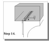
**Step. 7.** Drive the concrete nails into the bond beam 14" apart and 8" from the tile.
