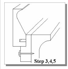
**Step 3.** Peel the paper from the double-faced tape (one foot at a time). Press the form to the ledger as illustrated.
