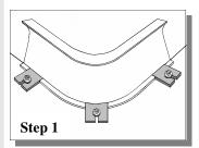
**Step 1.** Set the corners first. Make sure the string is hanging inside the step. Place a neoprene washer, neoprene side down on the screw. Drive the screw into the slot of the clip (as shown in step 1). Tighten the screw enough to hold the corner in place. Making sure the plastic clip can be removed later in the process.
