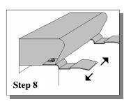
**Step 8.** Pull the form away. To remove the clips, wiggle them back and forth until the clips break loose, then pull them straight out.
