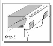
**Step 5.** While pouring, make sure to tap the forms to release air bubbles. This will help prevent honeycombing.
