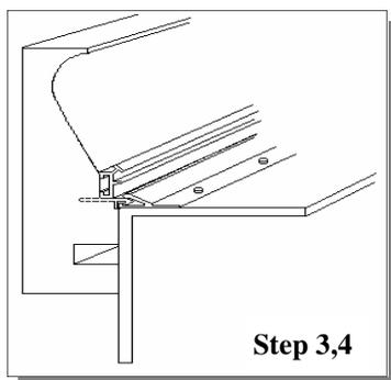
**Step 3.** Peel the brown paper from the double faced tape on the face of the form. Stick the fiber-optic receiver track (provided) to the face of the form.
