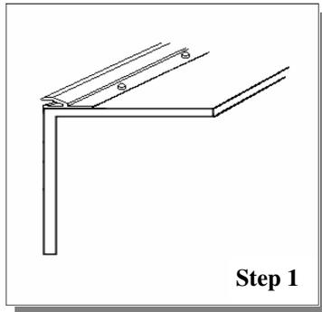
**Step 1.** Using the self tapping screws provided, attach the liner track to the top of the pool wall with the bottom of the track flush with the face of the panel. Space the screws approximately 14” apart, making sure the ends of the track are butted tightly together.
