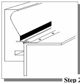
**Step 2.** Peel the brown paper from the double faced tape (one foot at a time) and attach the form to the panel pressing the rib of foam (just above the tapes) into the liner track. The plastic arrows embedded into the foam (at 6” intervals) snap into the track (with a snapping sound) by pressing against the back of the form with the palm of the hand.
