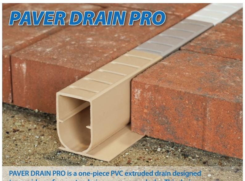
PAVER DRAIN PRO is a one-piece PVC extruded drain designed to provide surface water drainage on paver decks. This drain accommodates most 60mm or 2 %" height pavers.
